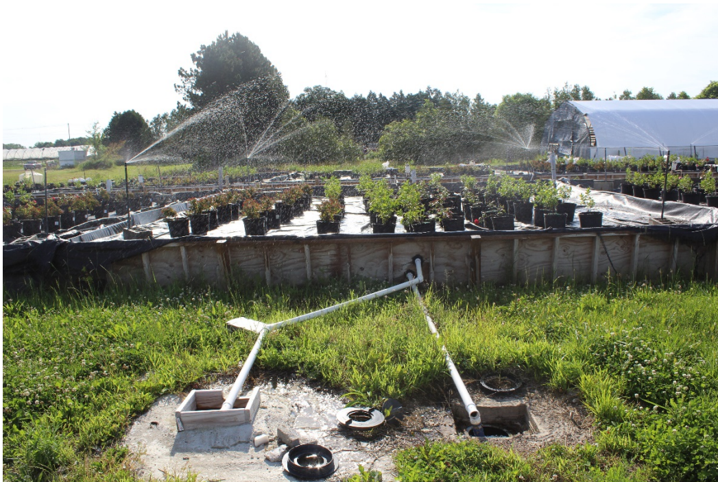
Image: One of the 16 raised beds, with surface runoff tank on the left and infiltration water tank on the right
