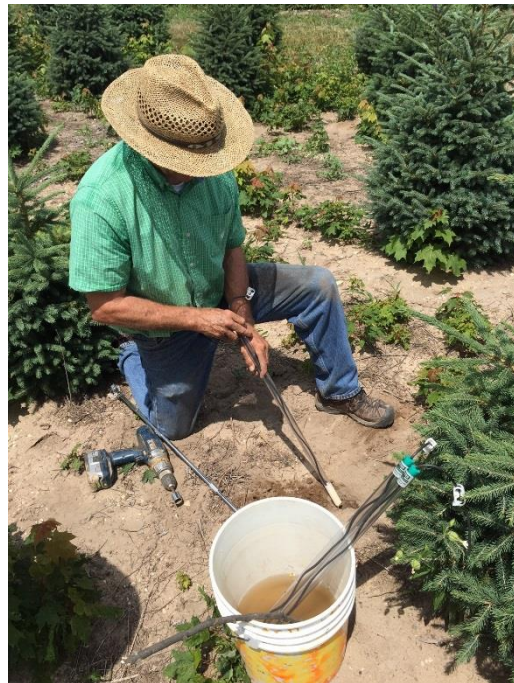
Lysimeter installation. Figure 2 (top) auguring pilot hole. Figure 3 (Right) inserting lysimeter sampling tube.
