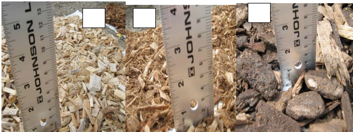
Fig. 19. Three bark types, (A) Hardwood bark (40% bark) (a composite of Oak, Poplar and Maple); (B) Cedar bark (bark and wood) (Eastern White Cedar); and, (C) Pine bark (70% bark) (a composite of White pine, Red pine and Jack Pine) obtained from Gro-Bark Ltd., Caledon, ON laid out approximately one inch thick before application of bio-herbicides.
