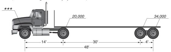
This combination has a bridge of 48' between axles 1 and 4. Using the B/F chart, this combination would be allowed a gross weight of 74,000 lbs. If the combination exceeds the B/F gross of 74,000 lbs., it would not qualify for bridge formula weights so only designated weights would apply (up to 18,000 lbs. on a single axle/16,000 lbs. for each axle on the tandem, with proper tire sizes).
