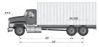
This vehicle has a bridge of 24' between axles 1 and 3. Using the B/F chart, this vehicle would be allowed a gross weight of 54,000 lbs. If this vehicle exceeds the B/F gross weight of 54,000 lbs., the vehicle does not qualify for the bridge formula so only designated weights would apply.
