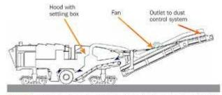
Figure 1: Asphalt pavement milling machine with silica dust controls (Nustration by NIOSH)
